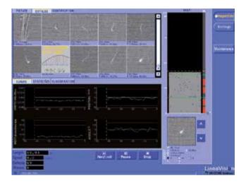
By continuously scanning the full surface, all defects are detected. A comprehensive and intuitive touch screen operator interface displays the inspection results and enables local configuration of the inspection station.
